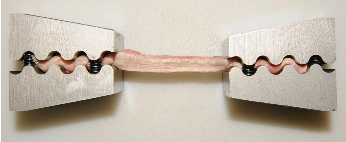
Figure 3 Specimen Mounted in the Wedge-Shaped Clamp Pads.
